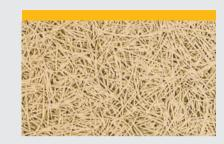
1-layer magnesite bonded wood wool acoustic panel (fibre width approx. 1 mm)
